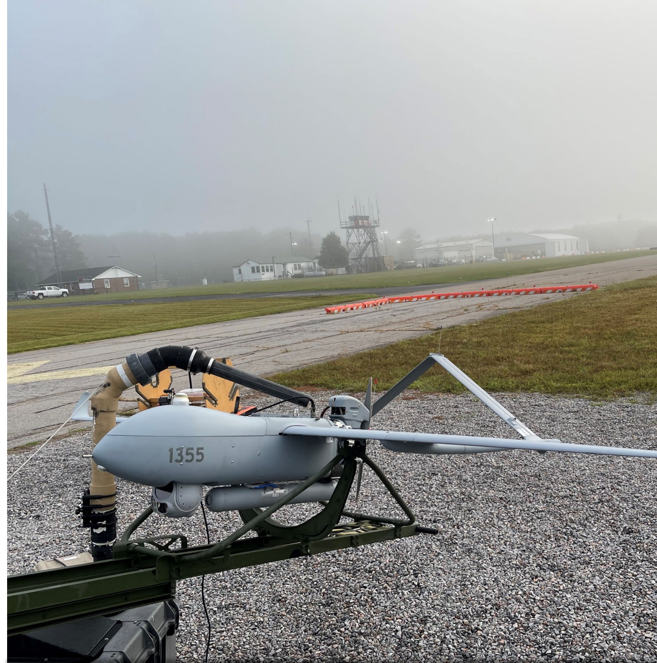
Aerosonde mk 4.7 with EO/IR sensor and SAR sensor
