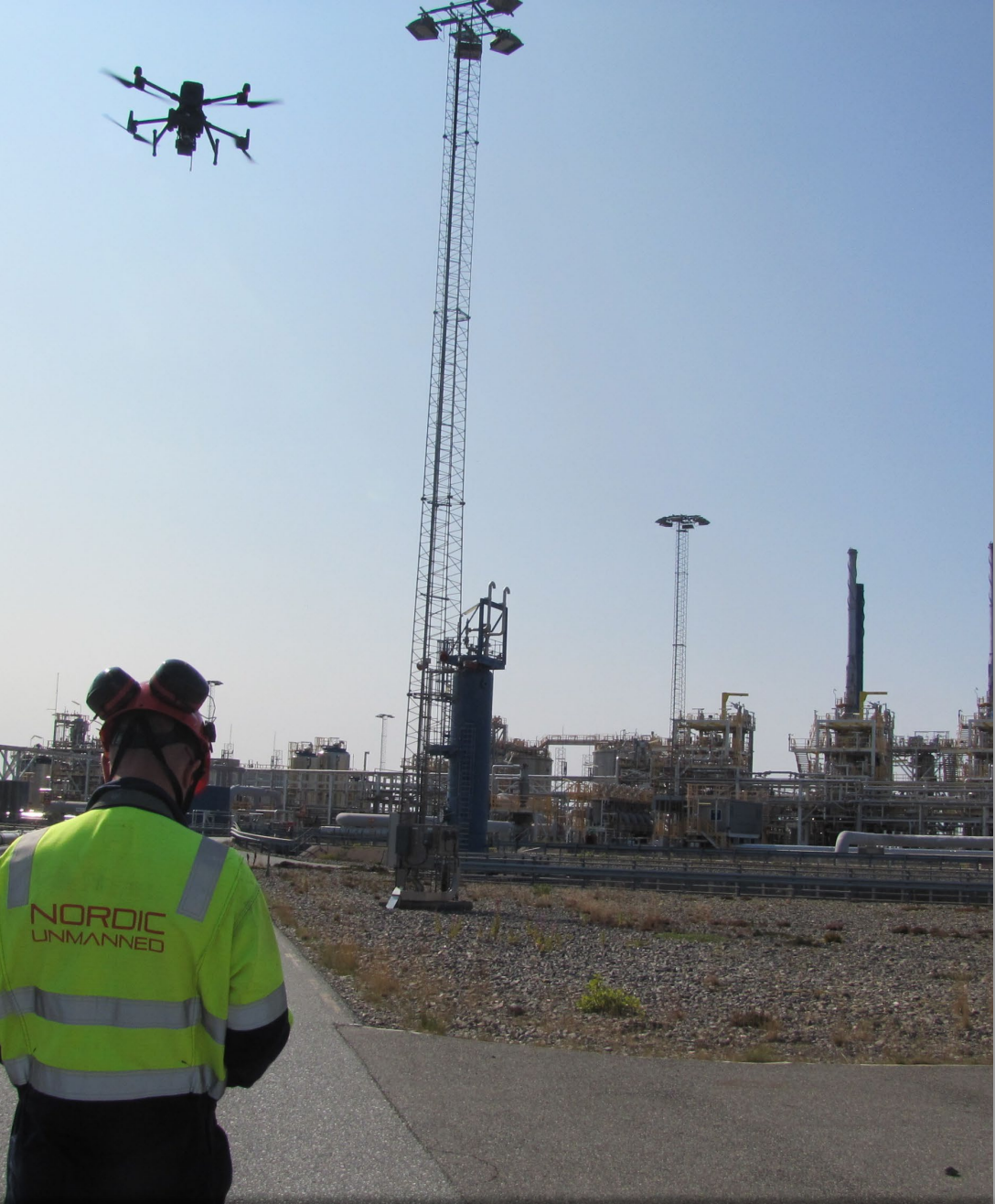
The Staaker BG-200 conducting methane sniffing with NUAer sensor
