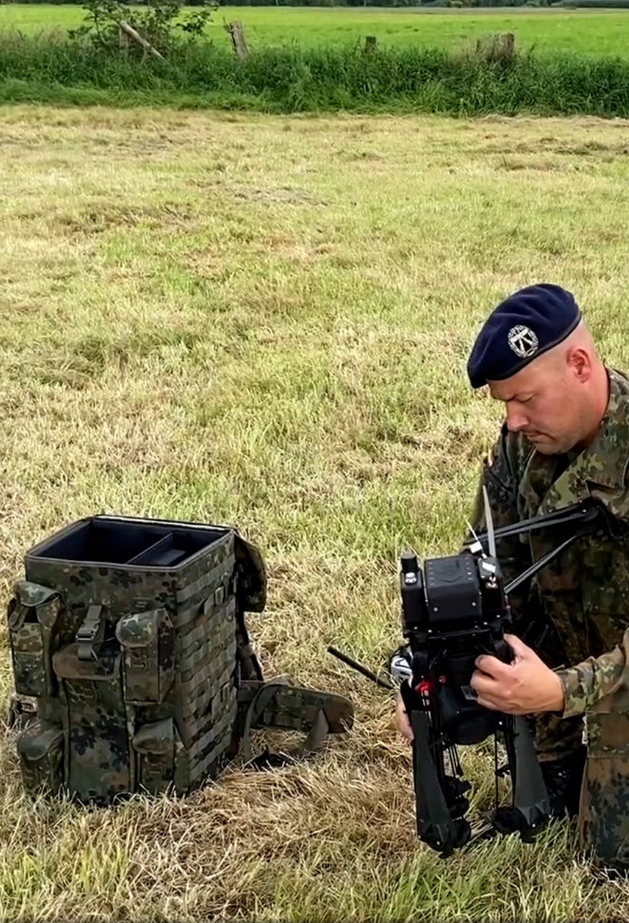
The AirRobot AR100-H being folded into its backpack
