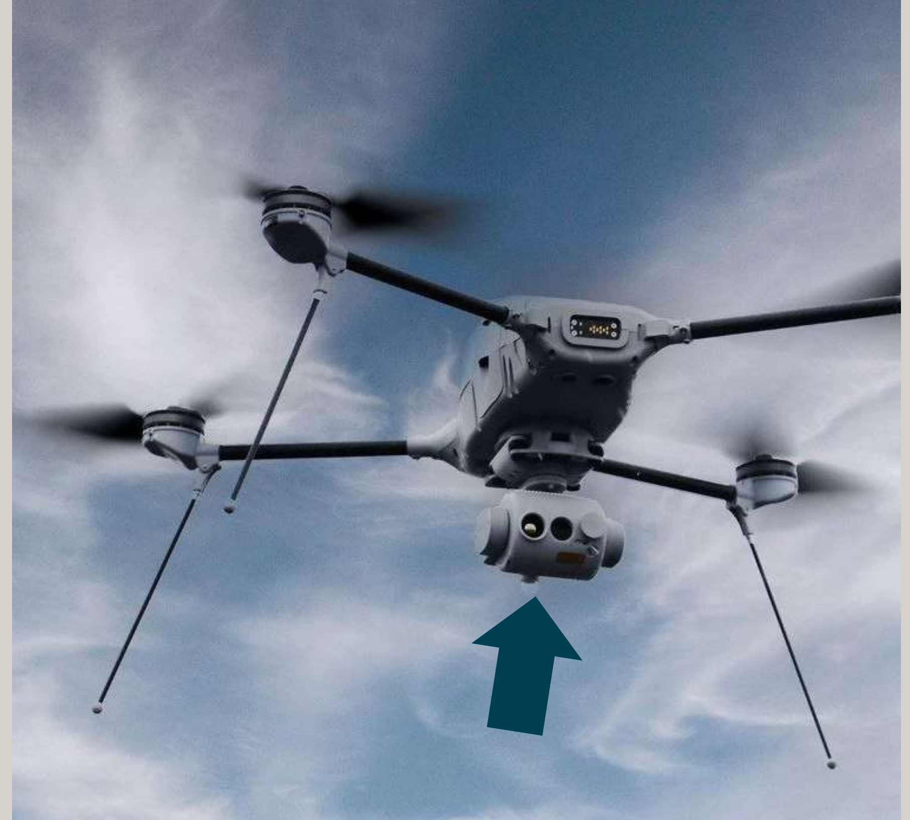
The Heimdal sensor mounted on a Lockheed Martin Indago 4
