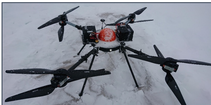
Figure 3: System with batteries mounted
